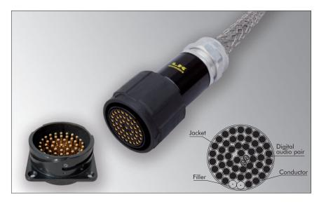
The **LKA 48/6** connector was designed to connect speaker clusters using as few cables as possible. It can carry up to 18 speaker and 2 AES/EBU channels with the **eurocable** 36N40AD2 cable or up to 48 speaker and 2 AES/EBU channels with the **eurocable** 48N40AD2 cable.
