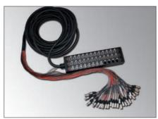
The SBF range features SSA cable (individually shielded multi-pair **eurocable**) hard wired to the XLRs in the box and an XLRs fan on the other end (available in various input and output combinations). The individual pairs are protected by Techflex to maintain ultimate flexibility. Use of coloured Techflex allows the easy identification of fan channels.
