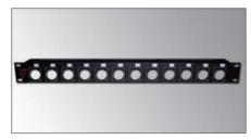
Pre-punched panels are available in a wide range of size configurations for easy and time-saving assembly of various types of connectors (XLRs, CEE form sockets, LK connectors). They are manufactured in 15/10 steel plate and finished in smooth black dust epoxy with silkscreen identification.
