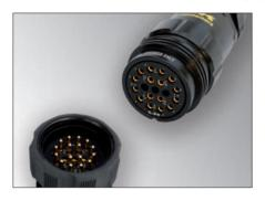
**LKA 16** (crimp pins) and **LKI 16** (solder pins) connectors are based on standard LKS Socapex style connectors but have been adapted to use only 16 pins, following indications from the largest rental companies. The standard Socapex style LKS 19 pin connector is also available, as utilized by D&B. Rubber locking ring available on both bayonet style and screw coupling connectors.
