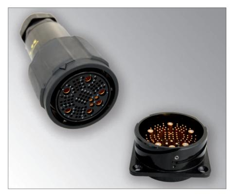
The **LKA 40/89** connector is the largest in the coax series and it features 80 pins size 18 for signal transmission, 6 coaxial pins and 3 pins size 12 for power.
