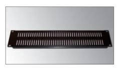
Specifically designed to give extra ventilation in the racks. They are manufactured in 20/10 aluminium plate finished in smooth, black dust, epoxy and have a 90° fold, top and bottom, to give better rigidity.
