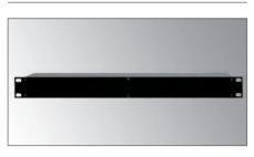
The front and the rear panel are manufactured in 30/10 black finished aluminium plate; they are available in 1, 2 and 3 rack units consisting of a "U" shaped base and top lid. They can be supplied customized with pre-punched and laser labelled holes on the front and rear upon request.
